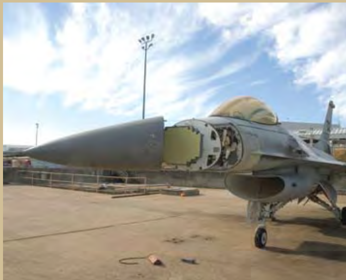
Figure 1 The Scalable Agile Beam Radar (SABR) installed in an F-16 fighter aircraft.
