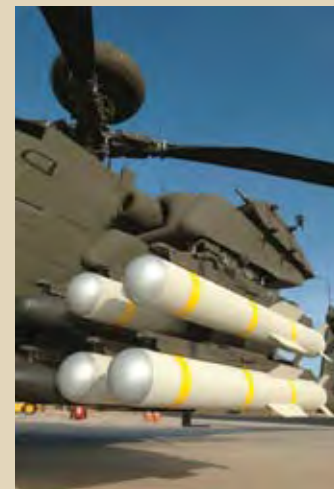
Figure 2 The JAGM features a Boeing body, a Boeing warhead and a Raytheon tri-mode seeker. The tri-mode seeker enables JAGM to attack a variety of fixed and moving targets regardless of weather conditions.
